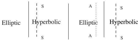
Fig. 17. Illustration of the nature of the three cases of elliptic, hyperbolic and mixed-type partial differential equations and the corresponding appropriate boundary conditions
